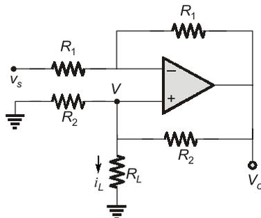
$$\frac{V}{R_2} + \frac{V}{R_L} = \frac{V_0 - V}{R_2}$$
