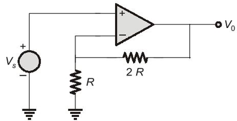
$$V_0 = \left(1 + \frac{R_f}{R_1}\right) V_s$$
